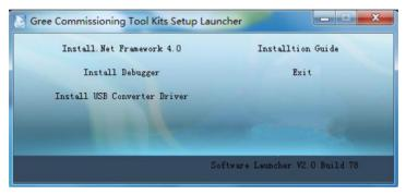
For the initial use of this commissioning tool kits, it is required to install .Net Framework 4.0, USB Converter Driver, and Debugger.
